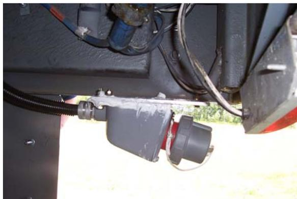
**Figure 3-2: Underside view of trailer plug assembly**
