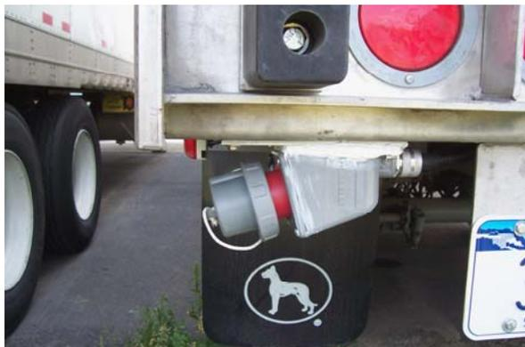
**Figure 3-1: Side view of trailer plug assembly**
