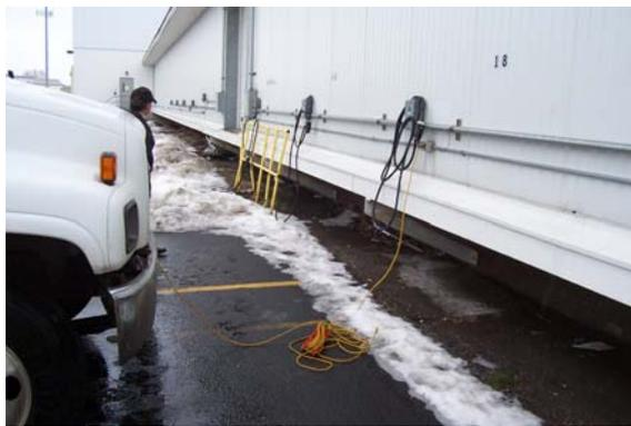
**Figure 1-2: Refrigerated box truck connected to electric power**
